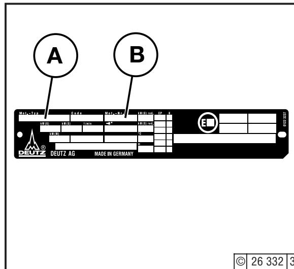
Engine model designation **A**, Engine Ser. No. **B** and the power rating are given on the maker's nameplate.
